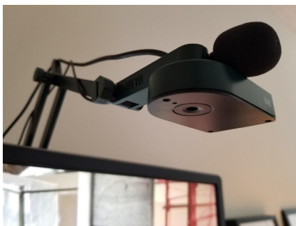
Fig.02 Overhead document camera allows for real-time sharing of materials located on the tabletop, including pencil/pen sketches, models, and printed reference books. Hand gestures can also be used to describe formal relationships, supplementing other modes of communication. Note that the microphone is sitting on top of the document camera, positioning the microphone within approximately 25cm (10-inches) of the mouth of the speaker, allowing for very clear audio. It is located just above (and outside) the field of view of the webcam.
